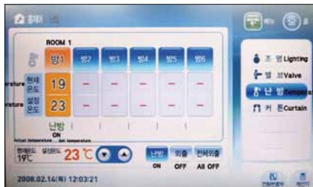
Comfortable operation of KNX functions by a central touch panel: for example, menus for heating, curtains and lighting.
