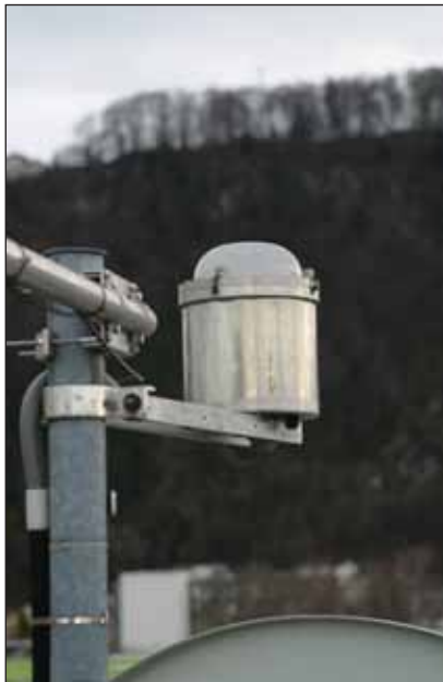
Picture 2: The heated metering box with light sensor
