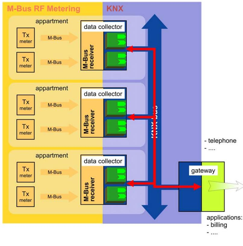
One KNX M-Bus Data Collector can receive, filter and interpret M-Bus Data of up to eight meters, each represented by a KNX Interface Object.
